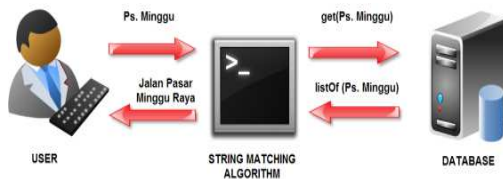
Figure 5. String Matching Algorithm Process
