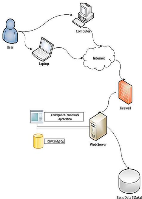
Figure 9. Deployment Diagram of SiZakat
