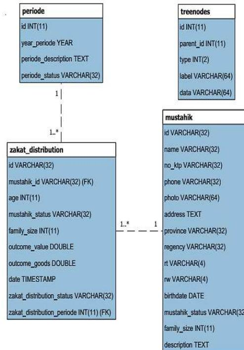
Figure 4. EER Diagram of SiZakat for addition feature
